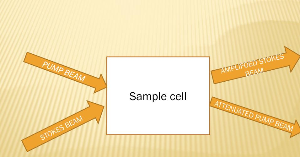
The frequency vs is tunable and satisfy the given condition. The incident beam with the frequencies i.e. pump beam and stokes beam interact with two energy states of the molecule.
